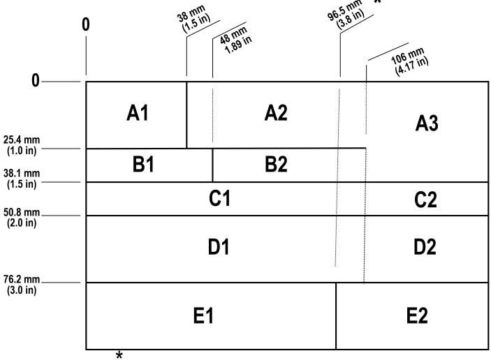
This dimension based on nominal 0.38 mm (0.015 in) Code 128 bar code license plate. The label provider must ensure quiet zone requirement of 6.4 mm (0.25 in) is maintained.
